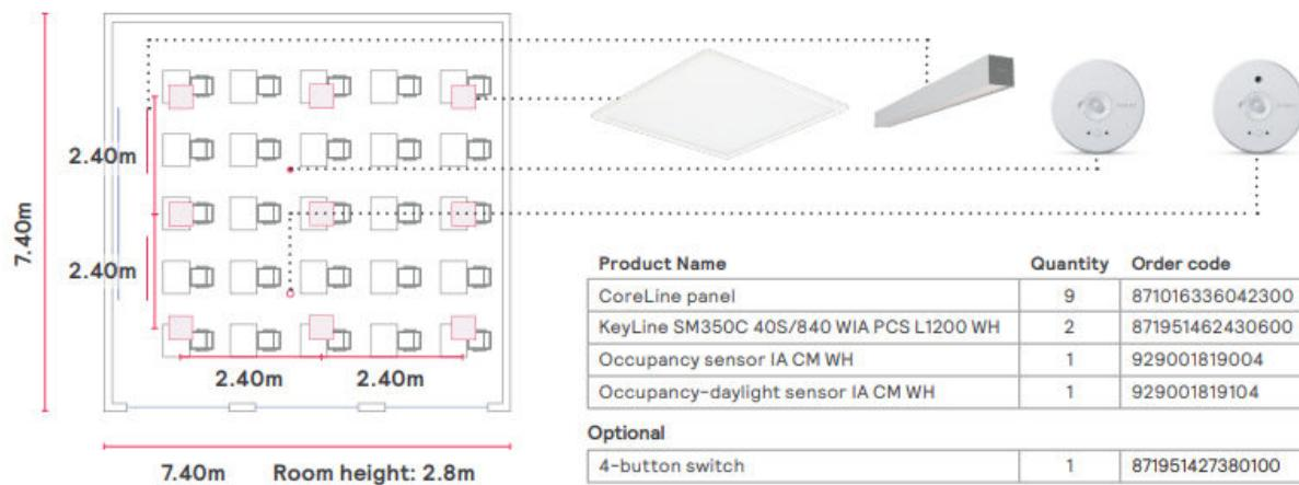
Classroom floorplan with a typical luminaire arrangement (sensor integrated in luminaire) \*
